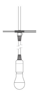
North America: E26, Max 60 Watts 120v AC 60hz
